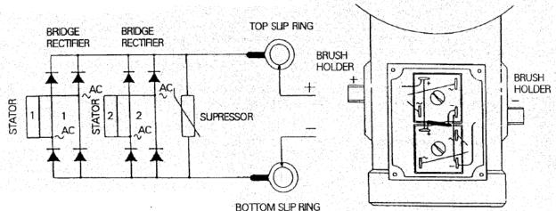
Figure 17: Ampair 100 Internal Wiring Diagram
