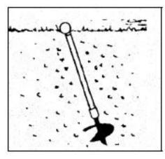
waterlogged soils which have poor holding and always anchor below the frost level.
