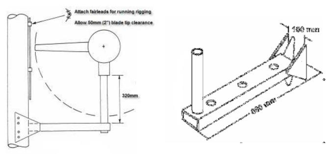
Fig. 9. Mizzen bracket mounting
