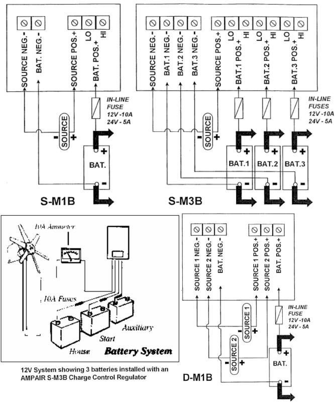
Figure 12. Charge Control Regulator - Wiring Diagrams
