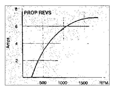
Figure 14: Ampair 100 Wind Generator Speed Curve
