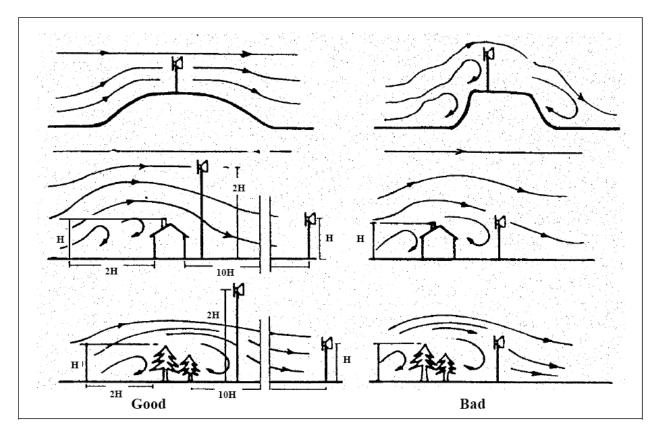
Figure 4: Wind Turbine Location Guides
