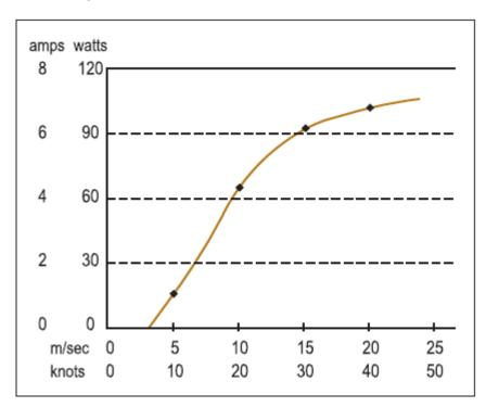
Figure 13: Ampair 100 Wind Generator Power Curve
